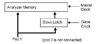
When the slave clock occurs, data captured on the pod is saved into the slave latch for the other pod in the *pod pair*. Then, when the master clock occurs, data captured on the pod, as well as the slave latch data, are saved in logic analyzer memory.
